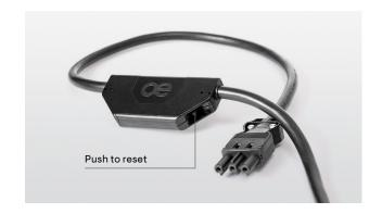
A thermal bimetallic strip, which has the advantage of being immune to high inrush currents and line transients, is heated by over current and deflects thereby releasing the latch mechanism. The contacts open even if the reset button is manually held in the closed position. This is known as trip-free mechanism. The contacts open and close with a positive snap action and the tripped state is clearly indicated by the extended projection of the reset button.
